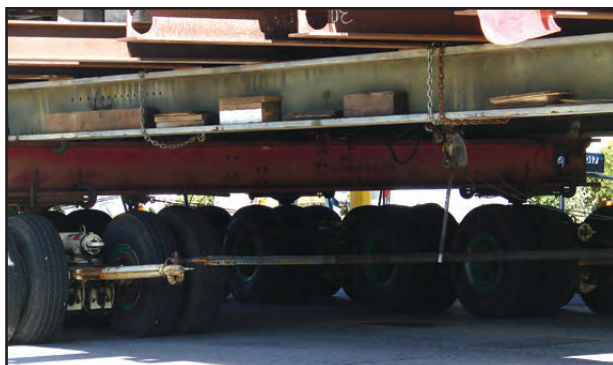
The suspension system adjusts to varying road contours to keep the house level and avoid cracking of interior walls during the move.
