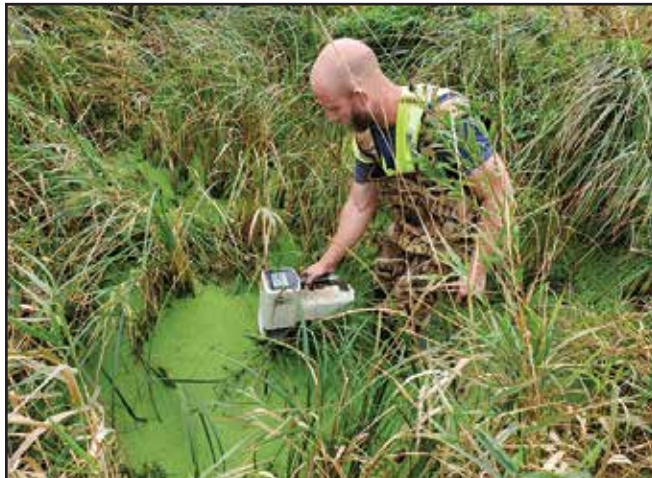
Technicians use imaging devices to check the position of the metal pipes used for boring. That sometimes means you're boring along the roadway (right photo) or even through a swampy area (photo on left). Crews are working hard to get as much boring and stringing fiber done before the ground freezes.
