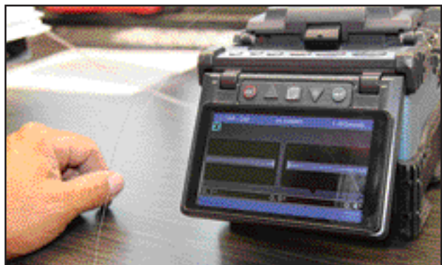
After each fiber has been cleaved at 90-degrees, the butt ends are aligned to prepare for the fuse. If the ends aren't cleaved, the splice would not be good and service may be compromised.
