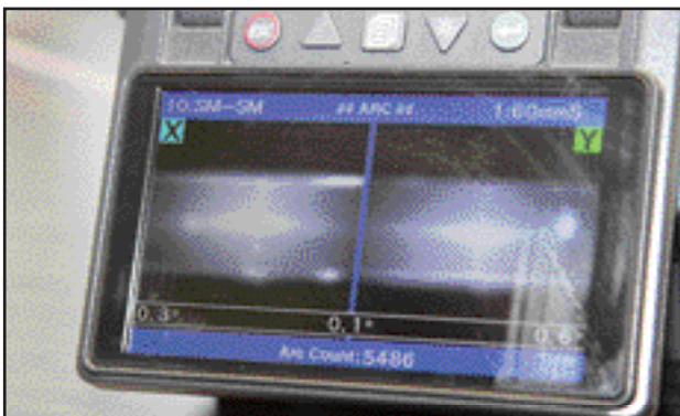
Cameras inside the splicing machine show the flash of the electrical arc that takes place during the splicing. The ends of both strands are fused.
