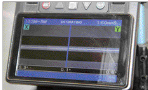
The cameras inside the machine show the finished splice. If it's done to specifications, the green "Y" is lit up. If not, the blue "X" lights up.
