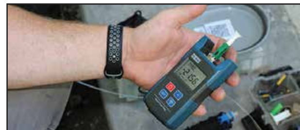
This meter checks to make sure the splice is good and the right amount of data is being conducted. Once the outside looks good, the technician continues to make connections to the router inside the home, checks that everything is working as it should, and answers any questions the homeowner has.
